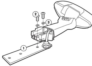
9. Put the sunvisor and the front mirror with the mirror extender with 6 press-in threaded screw (1). The screws must be adjusted in length so that the screws' thread engagement in the cab's weld nuts is the same as on the original sun visor.
