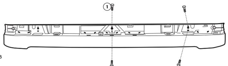
4. Place the bracket (2) on the respective LED-bar (1), with attached fasteners (3-6). Repeat and place the fasteners on the next LED-bar.
