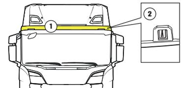
2. Disconnect the connector (3) between the cab and the front mirror (1) and remove the front mirror from the cab by removing 2 screws (2). Disconnect any contact piece for position lights between the cab and the sun visor. Remove position lights (4) with associated cabling from the sunvisor.
