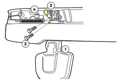
3. Remove the sunvisor from the cab by removing remaining 4 screws (1).
