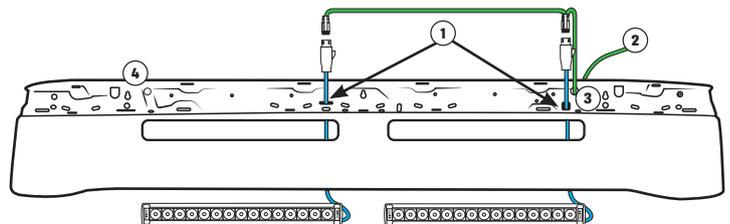
7. Pull 6 cable ties (1) from the back of the sunvisor through the pre-drilled holes and insert the wiring on the front of the sunvisor. Install any cabling for the position lights, use the pre-drilled ones the holes for cable ties if more attachment points for the wiring is required.
