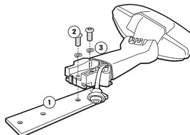
5. If equipped with position lights, fasten wiring to the position lights i new sun visor and use the pre-drilled holes for cable ties.
