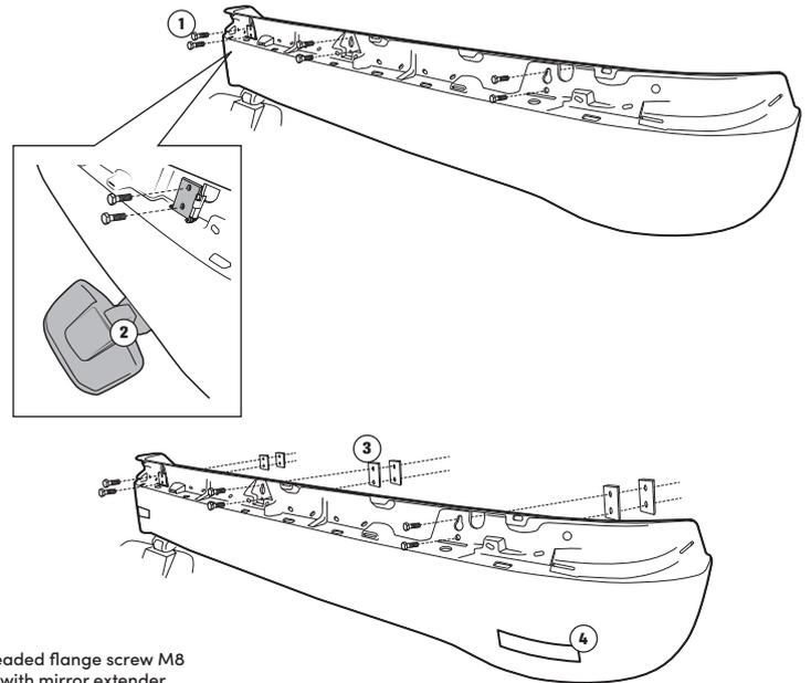
1. Press-in threaded flange screw M8
