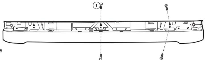
4. Place the mirror extender (1) on the front mirror with 2 screws (2) and spring washers (3)
